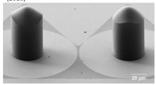
3D-printed lenses for coupling from a optical chip to a single-mode fiber (SMF). **a)** Lens on photonic-integrated circuit (PIC). **c)** Two anamorphic lenses on a SMF-array.
